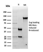
SDS-PAGE analysis of purified, BSA-free Interleukin 15 antibody (clone IL15/4353) as confirmation of integrity and purity.
