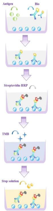
1. Add 50 μL standard or sample to the wells, immediately add 50 μL Biotinylated Detection Ab Working Solution to each well, incubate at 37°C for 30 minutes
