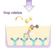
$5.\,Add\,\,50\,\mu L$  Stop Solution to each well. Read the plate at 450 nm immediately, calculation of the results.
