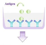
1. Add 100  $\mu L\,$  standard or sample to the wells. Incubate at 37°C for 90 min.
