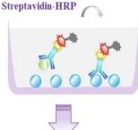
3. Add 100 µL Streptavidin-HRP Working Solution to each well, incubate at 37°C for 30 minutes, Aspirate and wash the plate for 3 times.
