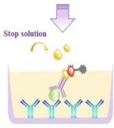
4. Add 50  $\mu L$  Stop Solution to each well. Read the plate at 450 nm immediately, calculation of the results.
