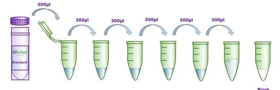
Notes: Store the zero tube with dissolved standards at  $2-8^{\circ}$ C and use it within 12h. Other diluted working solutions containing standards should be used in 2h.
