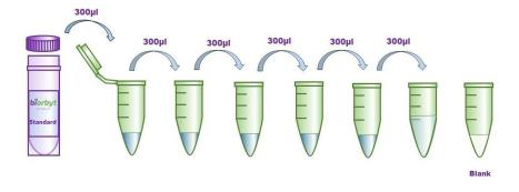
Notes: Store the dissolved **Concentrated standard** and **Zero tube** standard at 2-8°C and use it within 12h. Other diluted working solutions containing standards should be used in 2h.
