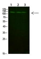
Western Blot analysis of 1,mouse-liver 2,hela 3,mouse-brain cells using primary antibody diluted at 1:1000(4°C overnight). Secondary antibody:Goat Anti-rabbit IgG IRDye 800( diluted at 1:5000, 25°C, 1 hour)
