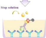
4. Aspirate and wash the plate for 3 times, add 100  $\mu L$  TMB Substrate Reagent to each well, incubate at 37 °C for 15~20 minutes.
