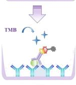
4. Aspirate and wash the plate for 3 times, add 100  $\mu L$  TMB Substrate Reagent to each well, incubate at 37  $^{\circ}C$  for 15~20 minutes.
