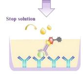
$5.\,Add\,50\,\mu L$  Stop Solution to each well. Read the plate at 450 nm immediately, calculation of the results.
