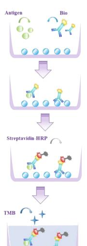
1. Add 50  $\mu L$  standard or sample to the wells, immediately add 50  $\mu L$  Biotinylated Detection Ab Working Solution to each well, incubate at 37°C for 30 minutes
