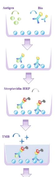
1. Add 50  $\mu L$  standard or sample to the wells, immediately add 50  $\mu L$  Biotinylated Detection Ab Working Solution to each well, incubate at 37°C for 30 minutes
