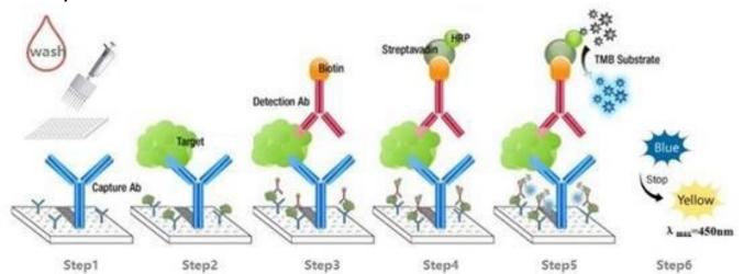
**Step1**: Wash plate 2 times before adding Standard, **Sample (diluted at least 1/2 with Sample Dilution Buffer)** and Control (blank) wells!
