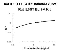
A standard curve is provided for demonstration only. A standard curve should be generated for each set of samples assayed.
