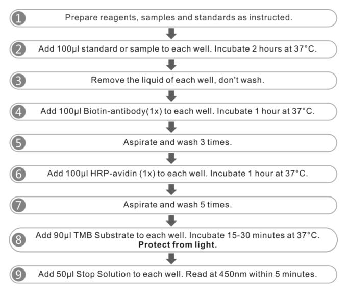
\*Please determine whether the sample needs to be diluted or the optimal dilution factor based on preliminary experiment result.
